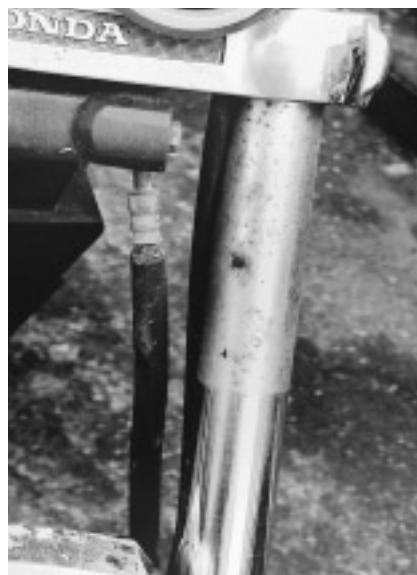
The corrosion on this fork tube makes it a sure bet no oil seal will last for long. The simple act of regular cleaning could have saved this owner hundreds of dollars in needed repairs.
